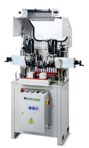
Knurling machine with manual axis positioning.
