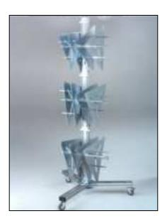
Decoiling trolley for rubber strips.
