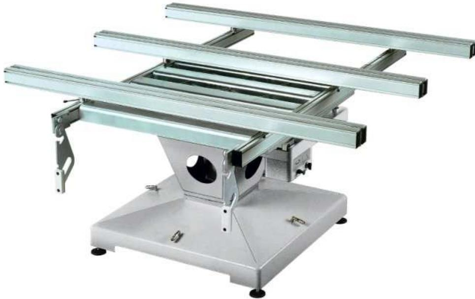
Extending, rotating and tilting assembly bench
