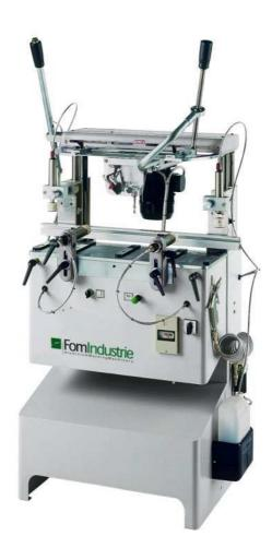
Electro-pneumatic copy router. The structure is realized by three principal monoblocs: bed in steel and heads units in cast iron. This solution is essential in view of the stress occuring during use. The machine is manufactured in accordance with CE regulation.
