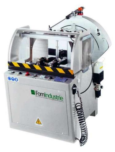
Single head sawing machine with  $\varnothing$  450 mm front blade and electronic cutting angle control. The machine consists of two large single block frames: the machine bed in normalised electro-welded steel and the cutting head unit in cast iron.
