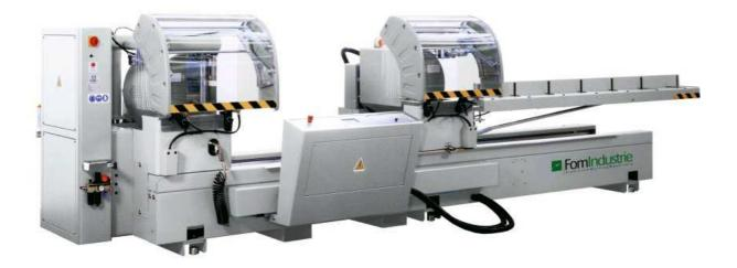
Double head sawing machine with  ${\it \varnothing}$  500 mm blade and electro-pneumatic cutting angle control
