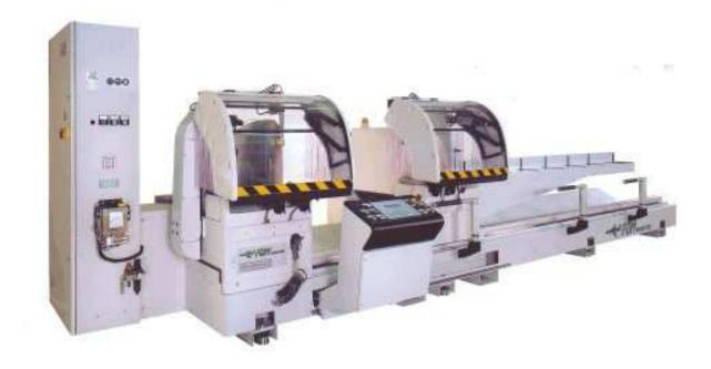
The machine comprises three solid structure single block frames, bed and bases, fixed and mobile head of a solid structure on electrowelded steel; kit support vertical vices and cutting area guard too; the tilting heads are in cast iron.
