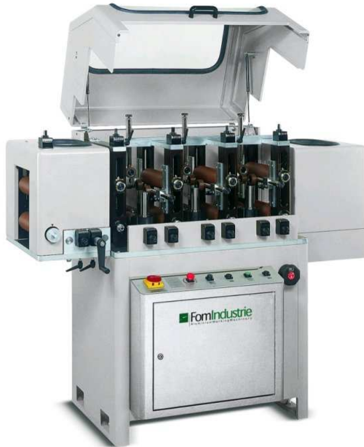
Roll-forming machine with manual axis positioning
