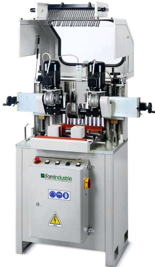
Knurling machine with manual axis positioning.
