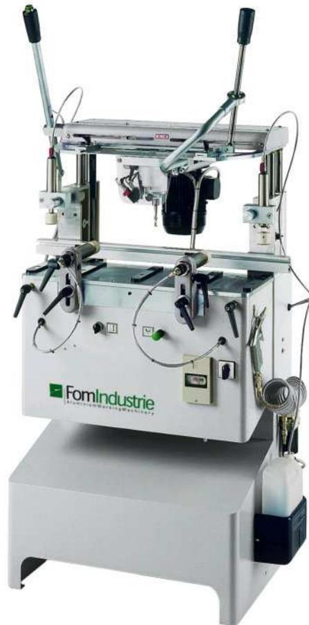
Electro-pneumatic copy router. The structure is realized by three principal monoblocs: bed in steel and heads units in cast iron. This solution is essential in view of the stress occurring during use. The machine is manufactured in accordance with CE regulation.
