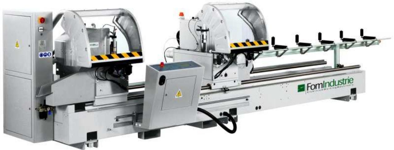
Double-head sawing machine with  $\varnothing$  500 blades and automatic positioning and electro cutting angle control
